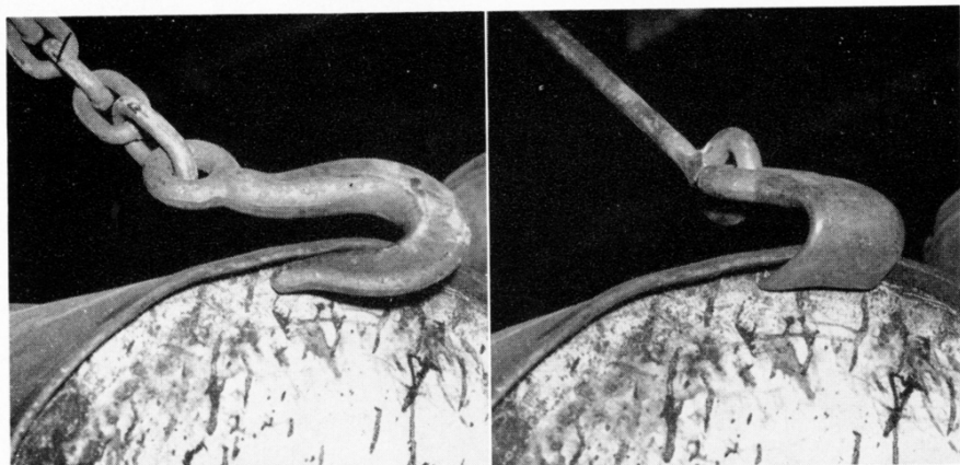
The right and wrong way to pick up a barrel. Left:—Wrong—The hook is insecure and the loading, being on its tip, makes it safe for only 41% of its capacity. Right:—Correct—A barrel hook with a sling made just for barrel lifting is used. One has never been known to have slipped or broken.
